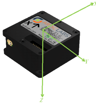
Figure 7: ArNav body coordinate system
